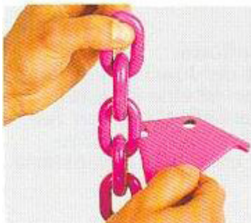
Testing wear of nominal diameter
