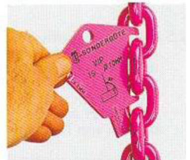
Testing plastic elongation caused by overloading
